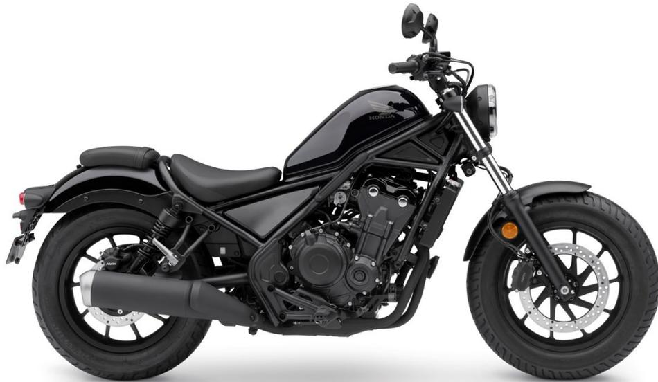
The Rebel, Honda's A2 licence-friendly 500cc parallel twin-cylinder compact cruiser benefits from revised suspension, full LED lighting, a new gear position indicator, slipper clutch and more comfortable seat. A new exhaust helps ensure Euro5 compliance.
